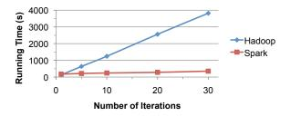
Figure 9: Hadoop and Spark logistic regression running times.
