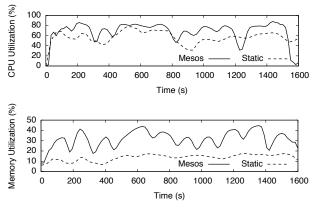
Figure 7: Average CPU and memory utilization over time across all nodes in the Mesos cluster vs. static partitioning.
