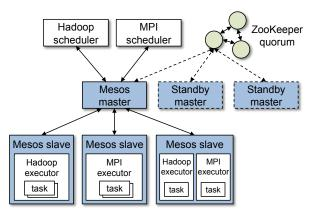
Figure 2: Mesos architecture diagram, showing two running frameworks (Hadoop and MPI).
